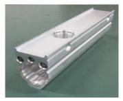
A door closer housing after machining
